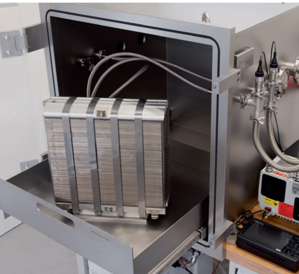
FIGURE 5 Fuel cell stack helium leakage measurement (© Dana)
